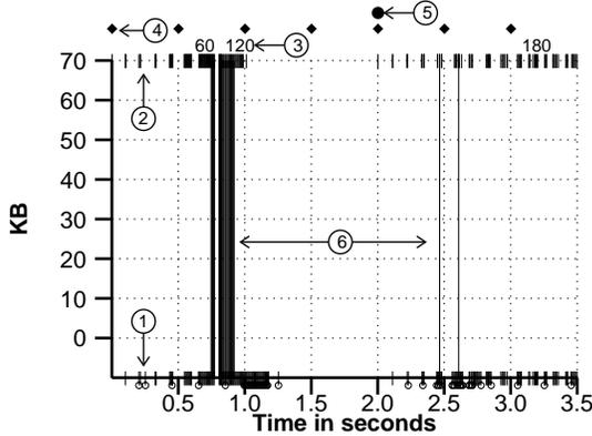
Figure 2: Common Elements in TCP Trace Graphs.
