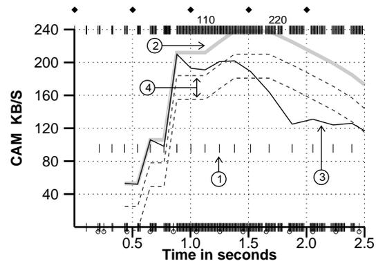
Figure 8: Congestion detection and avoidance in Vegas.
